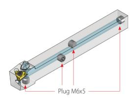
\* When reassembling the M6X5 plug, it is necessary to use LOCTITE 542.
