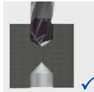
Breakthrough to bore in opposite direction; v_f = -50\%
