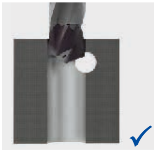
Bore off-centre; Chisel edge cutting
