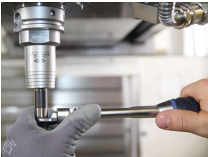
5. Note: Place your free hand on the replaceable milling head to be able to make delicate adjustments. This allows the tightening torque to be set more precisely. Tighten the replaceable milling head using the torque wrench and the corresponding open-end spanner at the specified tightening torque (see table "Tightening torque of replaceable milling head").
